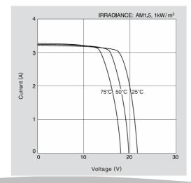
Current-Voltage characteristics of Photovoltaic Module KC50T-1 at various irradiance levels
