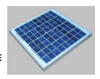
These modules are produces with high efficiency (>14%) polycrystalline solar cells made by Kyocera in Japan. These cells are encapsulated between a tempered glass cover and an EVA foil and TPE back sheet to provide maximum protection against severe environmental conditions. The entire laminate us installed in an anodized aluminum frame to provide structural strength and ease of installation. The junction box at the back is used for interconnection with other components of the system.
