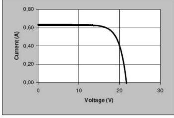
The electrical specifications are under test conditions of irradiance of 1 kW/m2, Spectrum of 1.5 air mass and cell temperature of 25°C. Minimum Power Output = Nominal Power - 10 %
