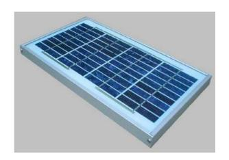
These modules are produces with high efficiency (>14%) polycrystalline solar cells made by Kyocera in Japan. These cells are encapsulated between a tempered glass cover and an EVA foil and TPE back sheet to provide maximum protection against severe environmental conditions. The entire laminate us installed in an anodized aluminum frame to provide structural strength and ease of installation. The junction box at the back is used for interconnection with other components of the system.
